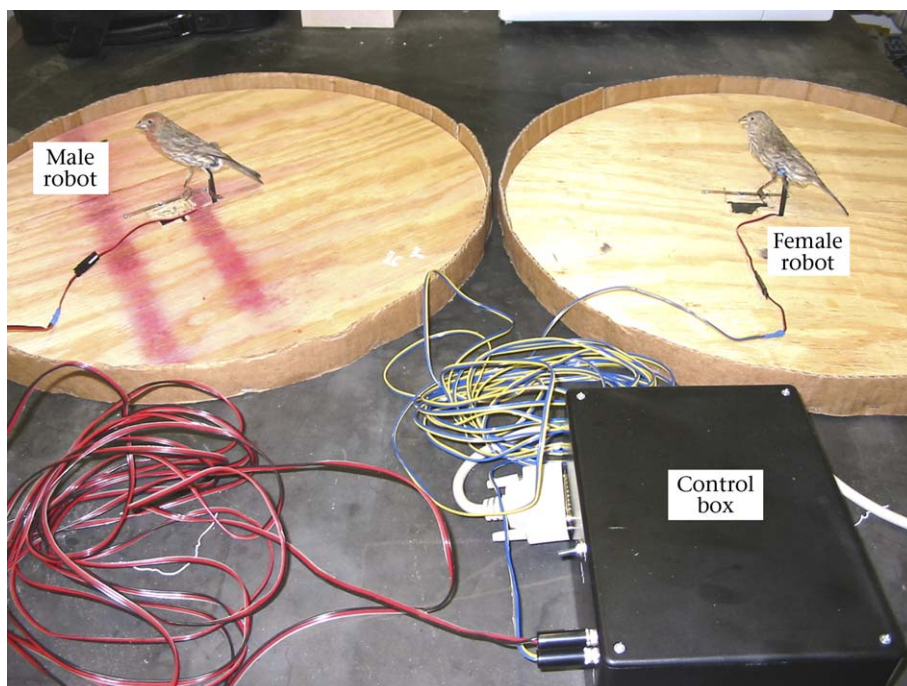
Figure 1. Robots used in the experiment built from male and female house finch skins. The picture shows robots in head-up position, the metal tubes that were used to pivot the robots, the wooded base of the enclosure without the bedding, and the control box that was connected to a laptop to control the frequency of head-up and head-down postures. This picture does not show the robots in the experimental set-up.
